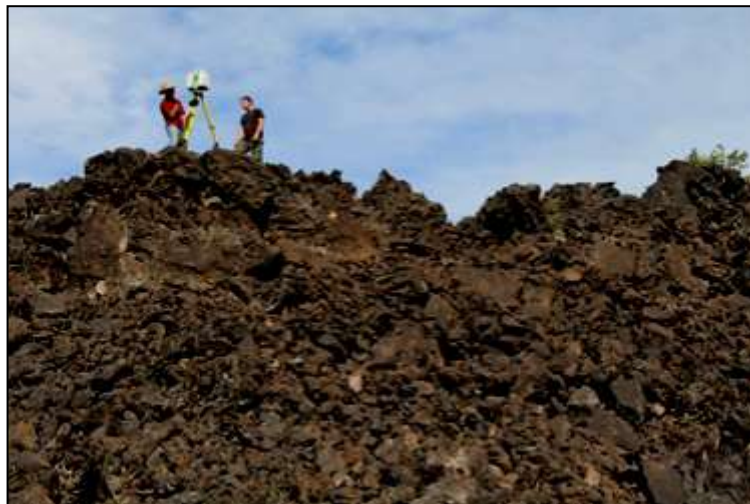
Undergraduate students Mike Barber and Drew Yetter set up the Leica terrestrial lidar scanner in order to scan the surface of the Mokst Butte lava flow in central Oregon.
