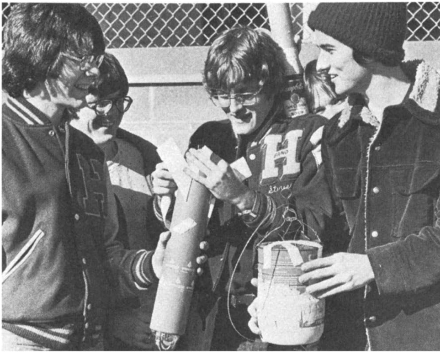
Fig. 4. Egg-Dropping Contest — Loading the egg into the drop container. At 15 to 20 m of drop height, limiting velocity problems begin to influence most designs unless very heavy containers are allowed. 1977 rules limit the container to several egg-masses and egg-lengths and a drop height of 10 m.
